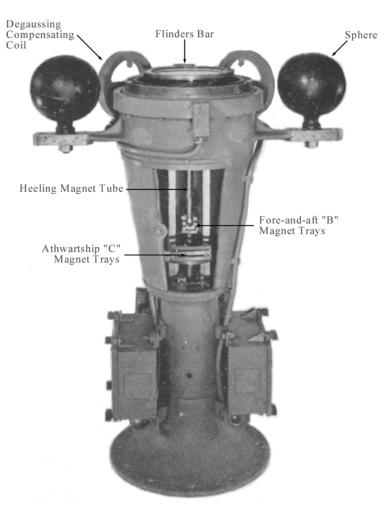
Figure 317 – Binnacle with compass and correctors
