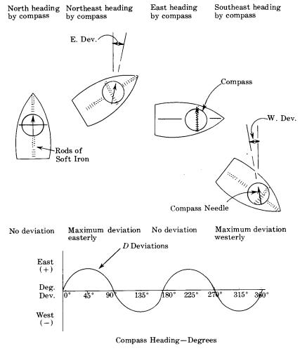
Figure 310 – Effects of symmetrical horizontal D induced magnetism
