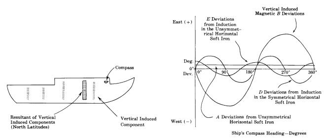
Figure 307a – Ship's vertical induced magnetism
