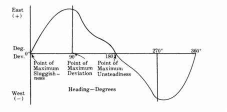
Figure 319 – Uncompensated deviation curve
