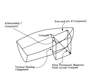
Figure 302a – Components of permanent magnetic field at the compass
