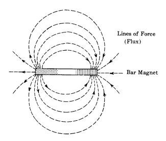
Figure 202 – Lines of magnetic force about a magnet
