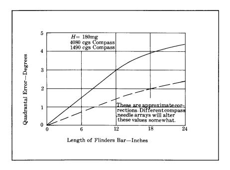
Figure 603b – Quandrantal error from Standard Navy Flinders bar.
