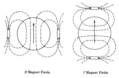
Figure 613b – Arrangements of corrector magnets
