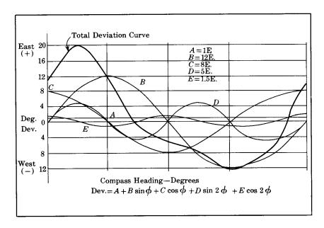
Figure 501 – Typical deviation curve and its individual components
