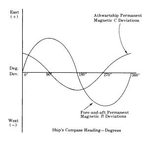
Figure 302b – Permanent magnetic deviation effects
