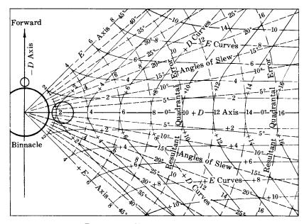
Figure 603a – Slewing of quadrantal spheres
