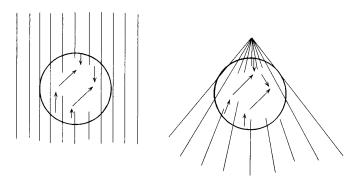
Figure 613a - Magnetic fields across compass needle arrays
