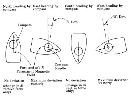
Figure 303a – Force diagrams for fore-and-aft permanent B magnetic field
