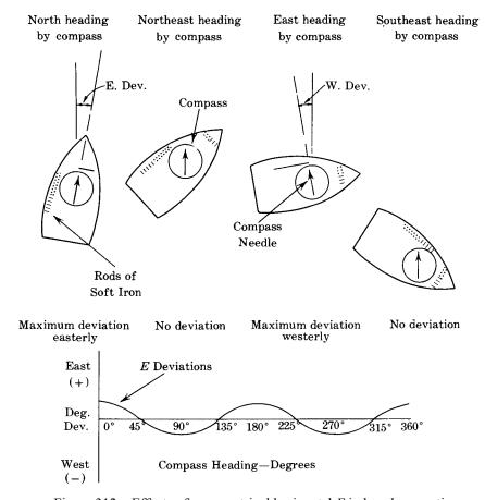
Figure 312 – Effects of asymmetrical horizontal E induced magnetism
