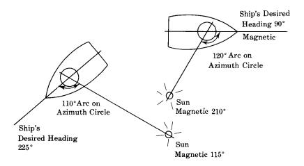
Figure 707 – Azimuth circle set-ups
