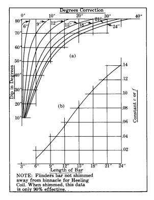
Figure 608 – Dip deviation curves for Flinders bar
