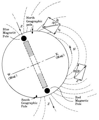
Figure 205 – Terrestrial magnetism
