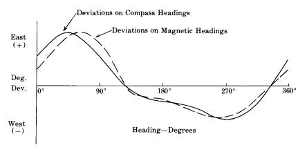
Figure 504 – Comparison of deviation curves (magnetic heading vs. compass heading).
