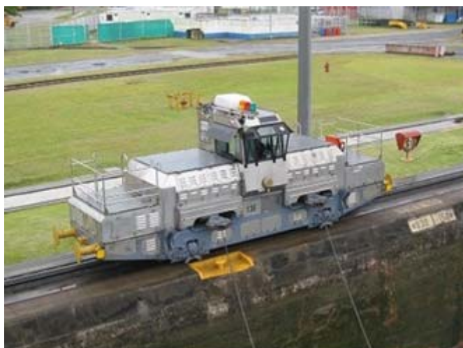
Electric locomotive (mule) used in original locks
