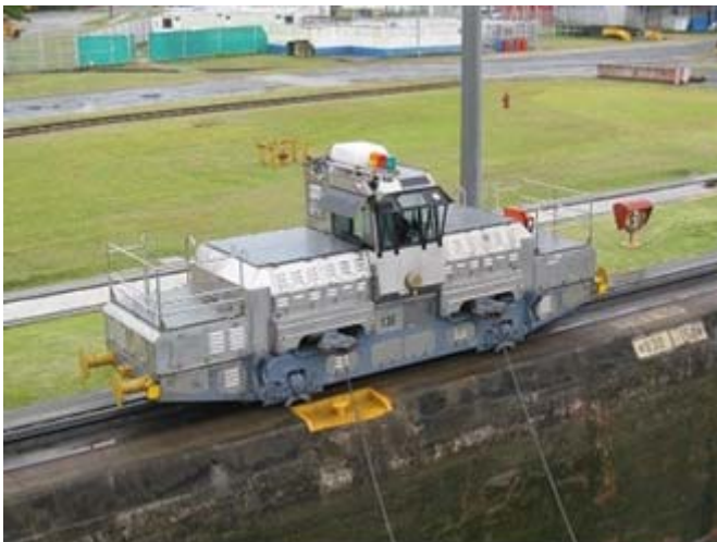
Electric locomotive (mule) used in original locks
