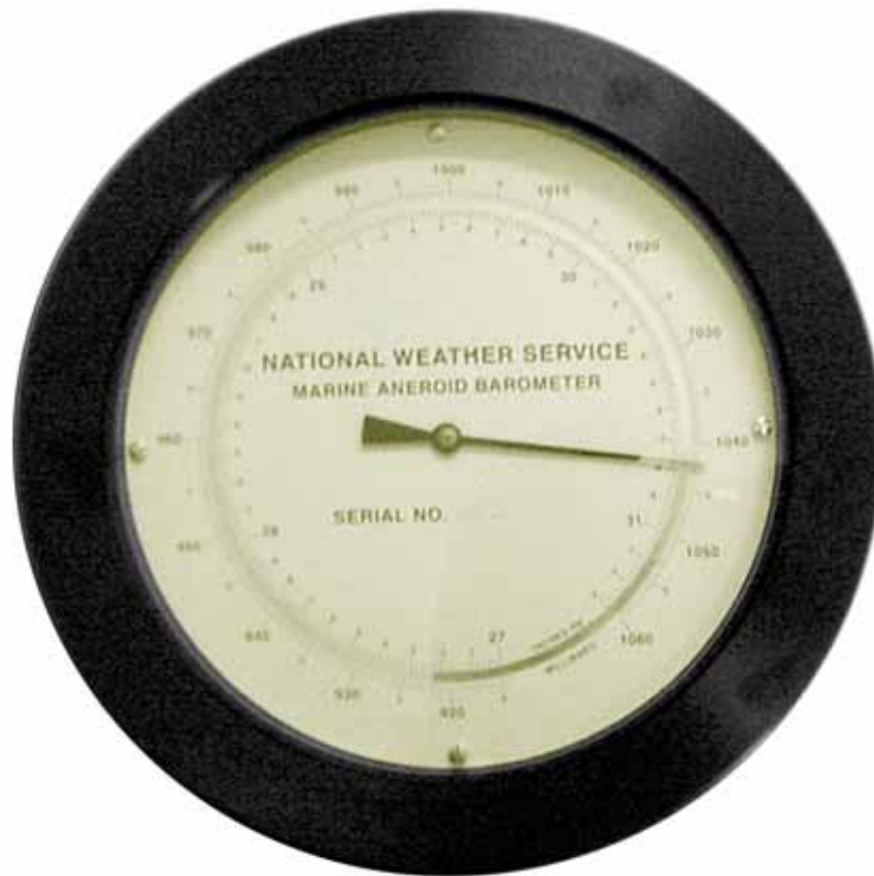
Figure 4002a. An aneroid barometer.
