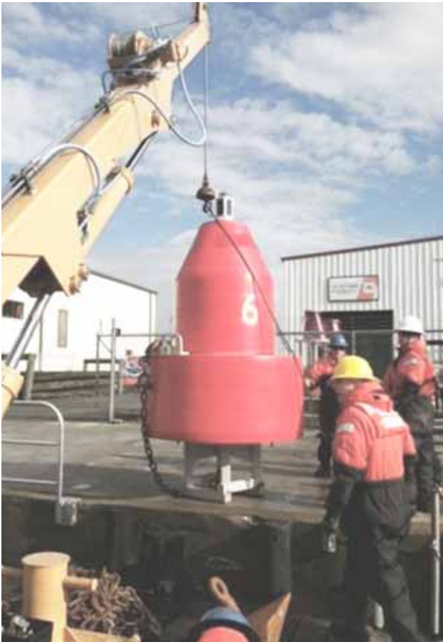
Figure 701b. Small lighted buoy.
