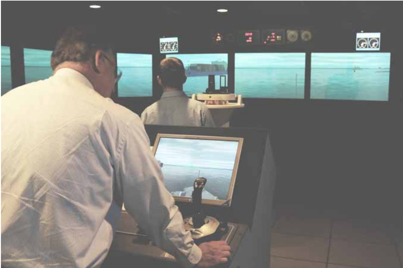
Figure 1025a. Navigational bridge simulator.
