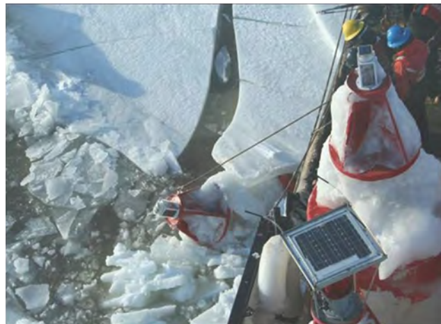
Figure 806. USCG recovering ice damaged buoys.
