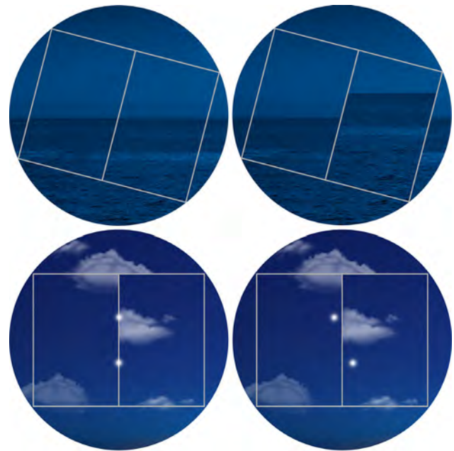
Figure 1511e. Testing the perpendicularity of the horizon glass. Left, side error does not exist. Right, side error does exist.
