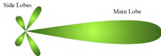
Figure 2406a. Freespace radiation pattern.
