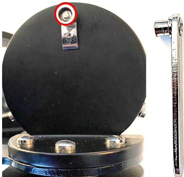
Figure 1511d. Adjustment port on the back of an index mirror and an adjustment wrench.
