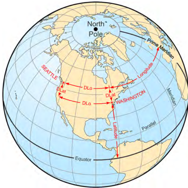
Figure F2b. Circles and coordinates on the Earth. All parallels except the equator are small circles; the equator and meridians are great circles.
