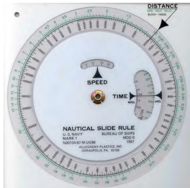
Figure 501b. The nautical slide rule.
